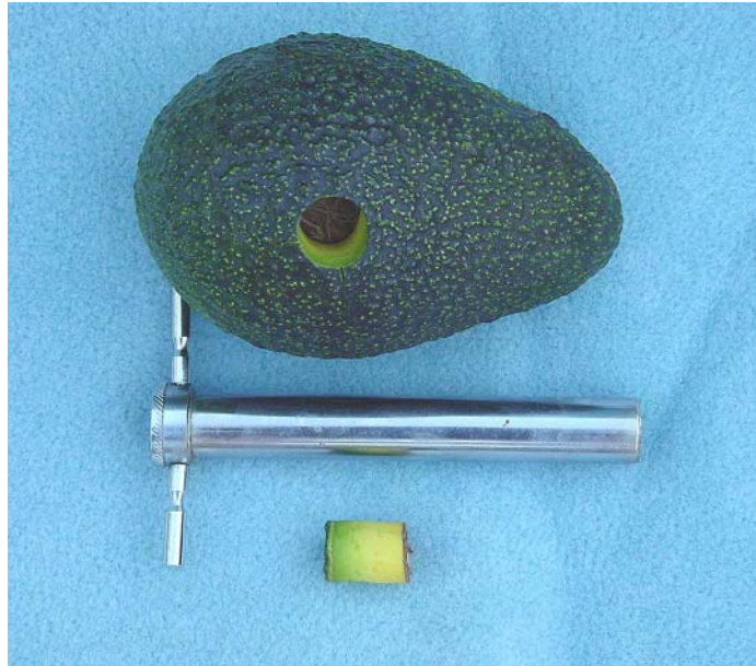
Figure 8. Core sample using a hand held coring tool.
